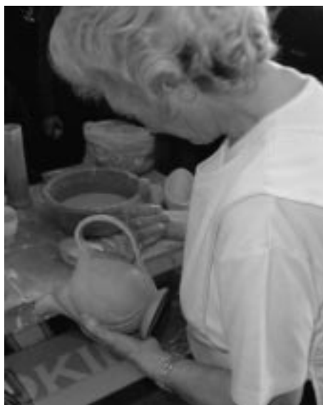
Seen on the day... "Fettling", demonstrated here by Vi Spearman, means smoothing off the piece after it emerges from the mould. A knife or other sharp blade would be used to remove the ridge of clay which occurred where the two halves of the mould met. Handles would be fettled by hand and with the help of a "pegger" (a small, rounded stick).
