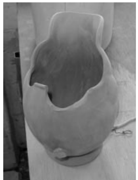
Seen on the day... Here's what happens when you pass a "green" pot around some forty members who aren't used to handling them. And this was one of the previously-cast pieces which had been in the mould for two days. Remember what we said about delicacy of touch? The fettlers would be taking pieces out of the moulds after only half an hour or so. And, needless to say, they wouldn't have been paid for a piece in this condition!
