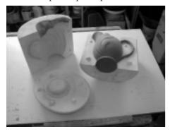
trough and recycled. The moulds were then placed in a mould chamber where the slip was dried through the action of gas burners. Each mould had a life-span of a hundred and twenty fillings. While it was drying, the clay piece contracted and could be removed when the mould was opened.
